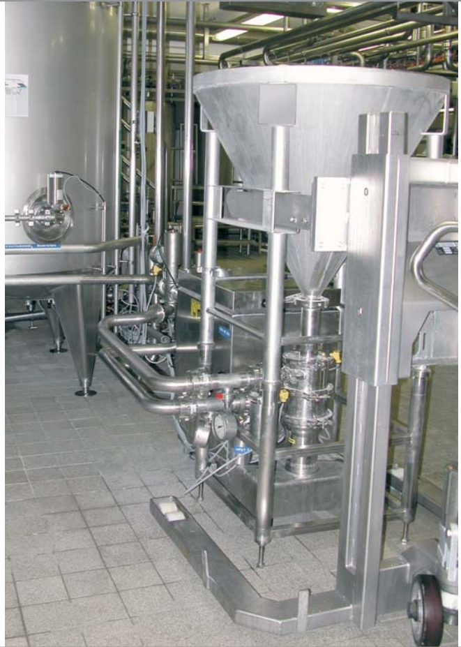
YTRON-ZC in the Dairy Industry Application: Dispersing of Stabilizer for the production of drinking yoghurt
