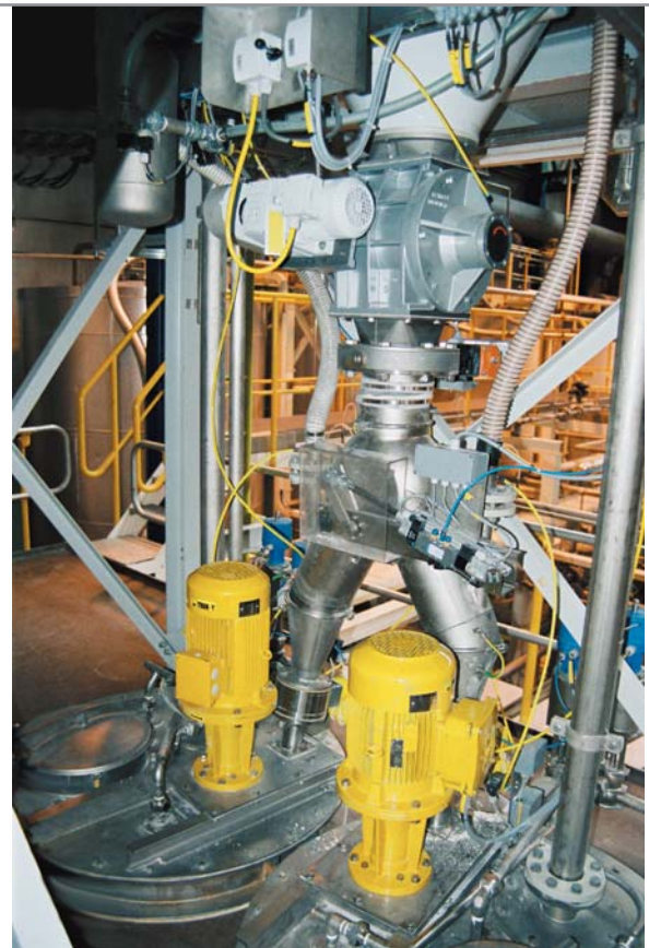
YTRON-Y ByPass in the Brewing Industry Application: Suspending of Diatomaceous Earth CO 2 inerting for a Continuous Discharge of the Product
