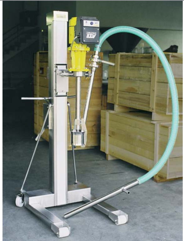
YTRON-Y with ByPass on a Mobile Hoist
