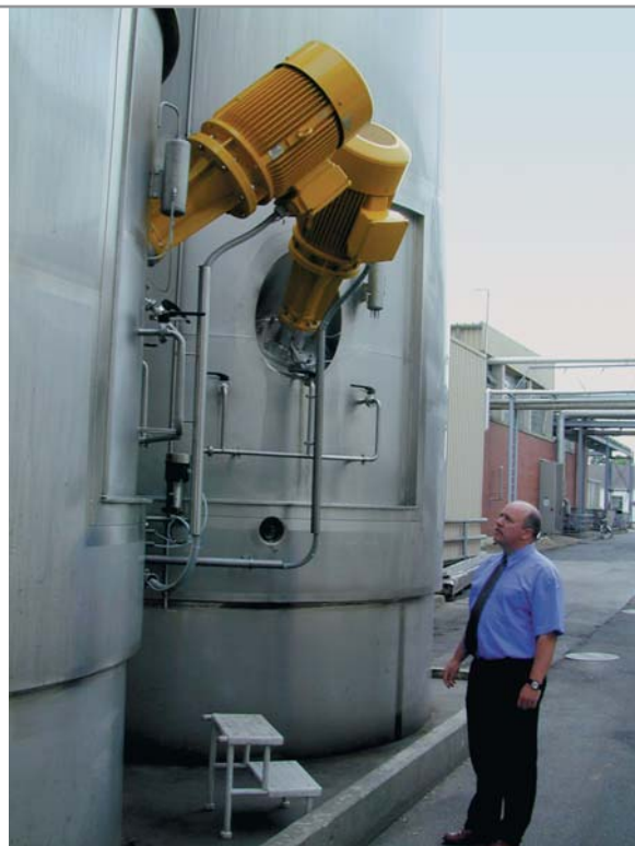
YTRON -Y in Side Entry Tank-flange execution below Liquid Level Application: Fermented Milk for Fromage Frais Production (100.000 litres capacity)
