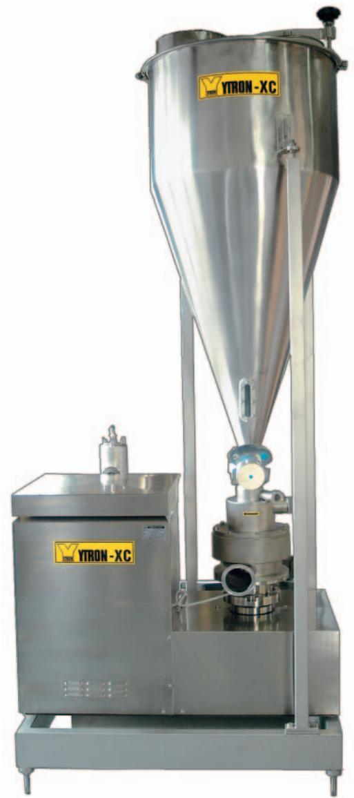
YTRON-XC with special hopper for connection to a powder feeding system
